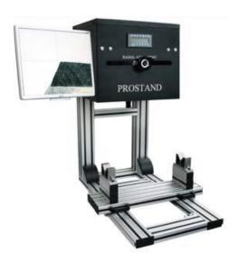
ProStand HD is a system for measuring, calibrating and cataloging woodworking machinery cutterheads. The ProStand system hardware is a two-axis cutterhead setup stand that allows an operator to digitally measure cutterhead radius, axial position, length of arcs, arc center points, arc radius, knife alignment and more. It makes non-contact, digital measurements using a color CCD camera coupled to a magnification lens, a high resolution 17" LCD color monitor and ProStand digital read out.
